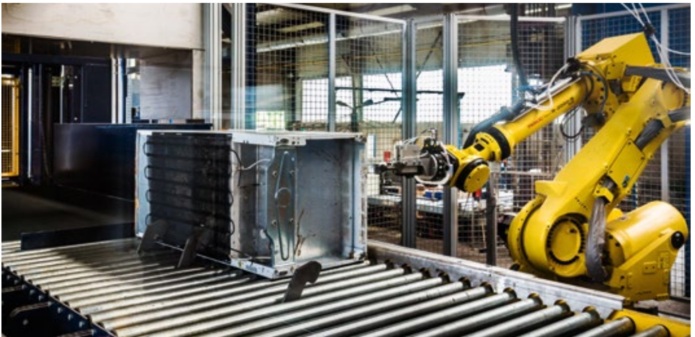
Pentane or CFC? The test result from the measuring robot determines the recycling unit to which the refrigerator is sent.
