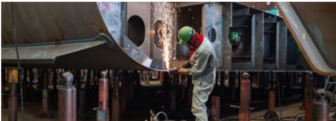
Components are cut to size with blowtorches and taken to the steelworks, where they are heated and rolled into sheets.
