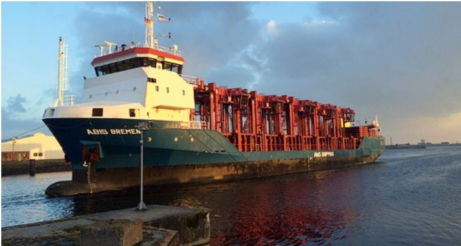
Impressive dimensions: each container straddle carrier is 15 metres high and weighs around 70 tonnes.
