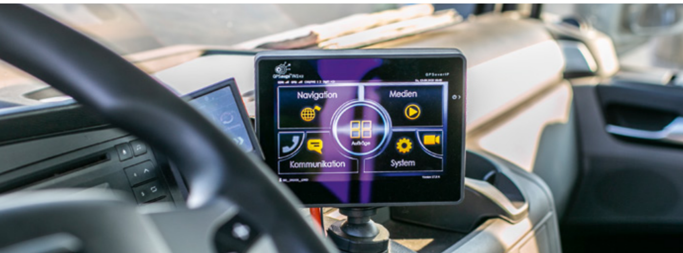
Intelligent networking: The telematics system in waste disposal trucks communicates with skips.
